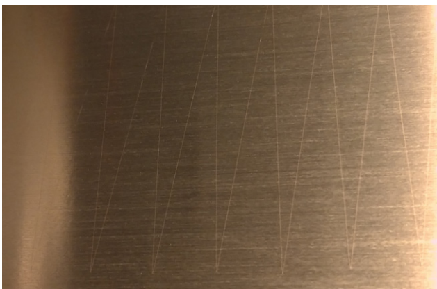
Fig. 4: Zigzag pattern on Cu substrate in continuous coating machine
