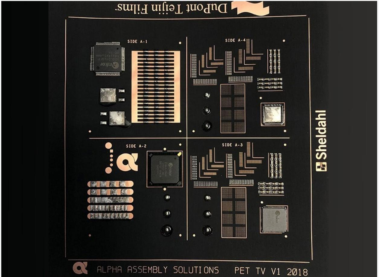
**Black PET film for Flexible Printed Circuit (FPC) boards**
