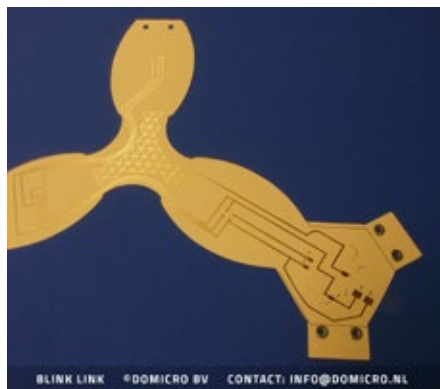
Fig. 4: Flexible LED ball by folding 2D printed electronics on paper into a 3D shape
