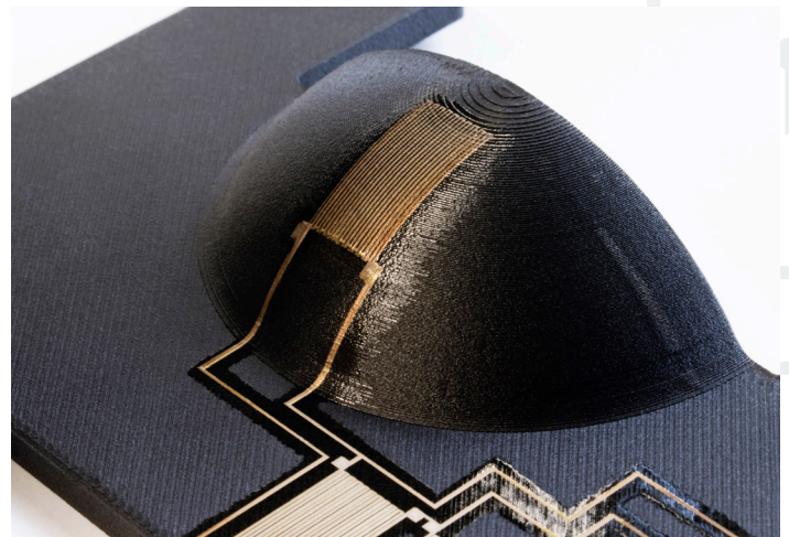
Conformal aerosol-printed strain gauge on top of aerosol printed dielectric
