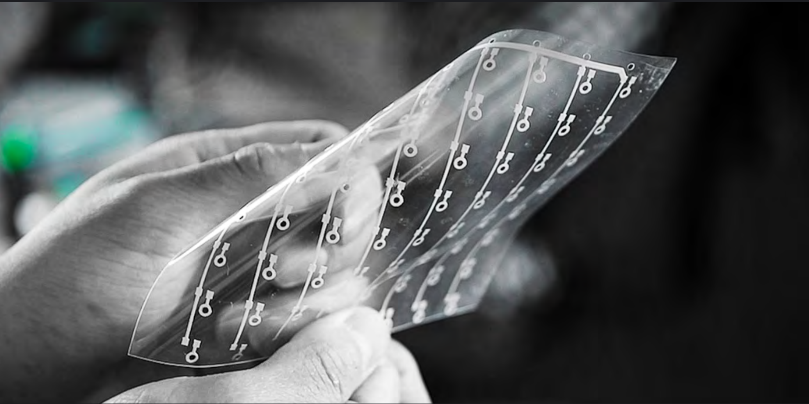
One panel of a transparent 8x8x8 LED matrix. Traces printed and eventually solder paste dispensed by the Voltera V-One.
