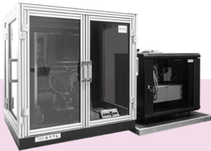
XTPL® DELTA PRINTING SYSTEM high-precision rapid prototyping printing system for microelectronics
