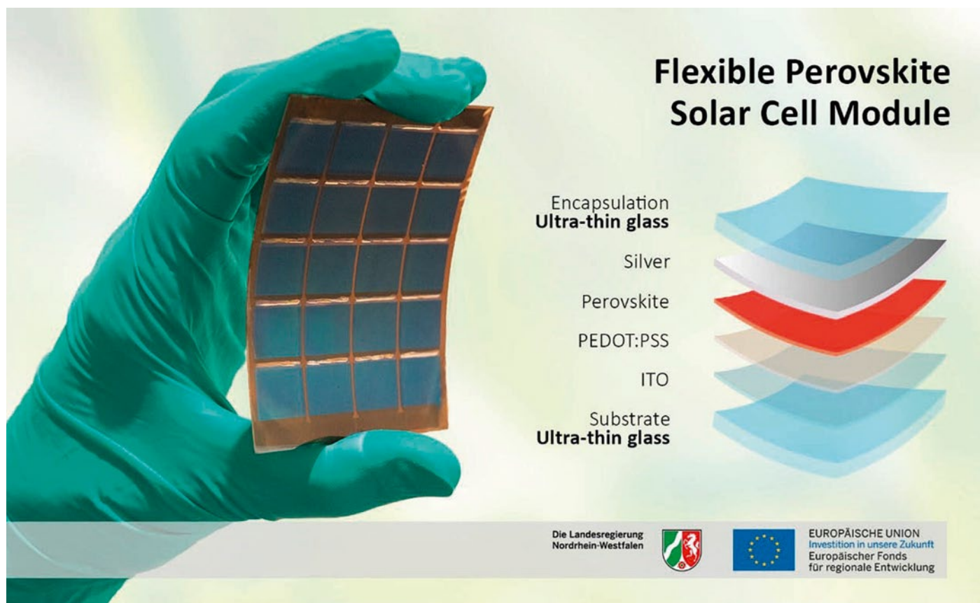
Figure 3: Flexible perovskite solar cell demonstrator using ultra-thin glass and a schematic illustration of the used device stack.
