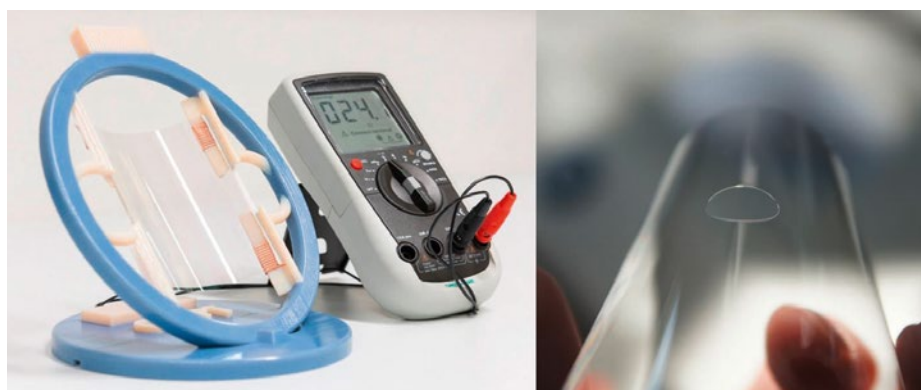
Figure 1: ITO-coating on ultra-thin glass (left) and cut structure in ultra-thin glass (10mm in diameter) (right).
