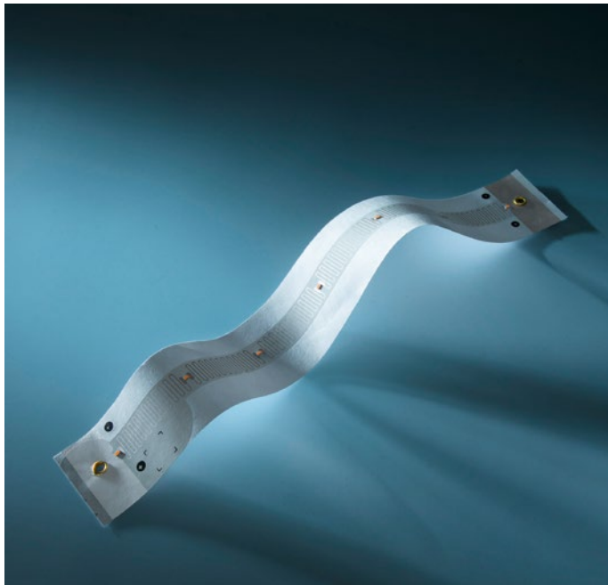
Fig 2: A lightweight – this segment (50x350mm) contains seven LEDs and weighs about 2 grammes
