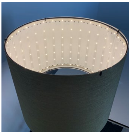
Fig 1a: A flexible LED board made of paper combined with a décor layer results in an innovative approach for a lampshade
