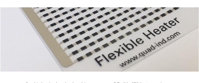
Quad Industries has developed its own range of flexible PTC heaters, using our expertise in printed electronics. The Positive Temperature Coefficient (PTC) functionality enables **self-regulation** to a specific temperature, offering **uniform and flexible heating** while increasing **safety**. Quad Industries helps you explore the different possibilities of new flexible heating technologies and guides you from the initial idea to the finished product.
