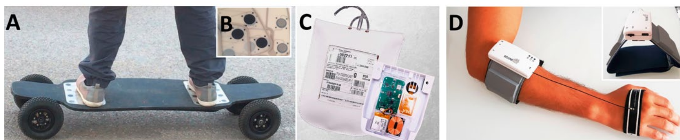
SmartEEs Application Experiment prototypes: ETS – Pressure sensor controlled e-skateboard (A) with printed pressure sensors; BOSET – Blood transfusion monitoring device for cold chain maintenance (C) ; RFLEX - Radio frequency based flexible care for rehabilitation (D)
