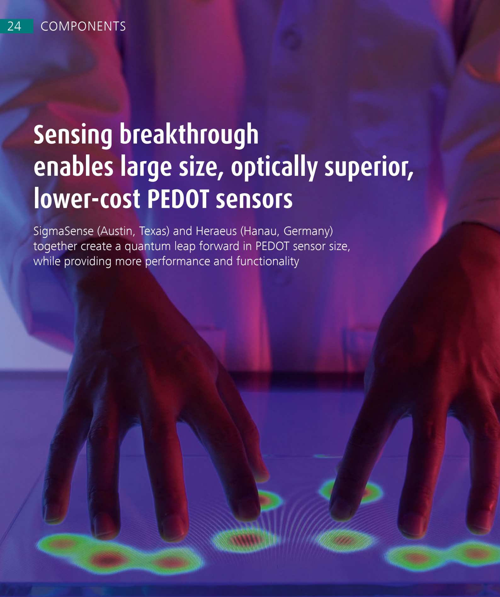
Fig 1: Heraeus PEDOT-based 65-inch high resistance sensor demonstrates a lower cost, optically superior touch sensor manufactured by TWS. SigmaSense's SigmaDrive technology enables using the high resistance touch sensor while providing breakthrough performance
