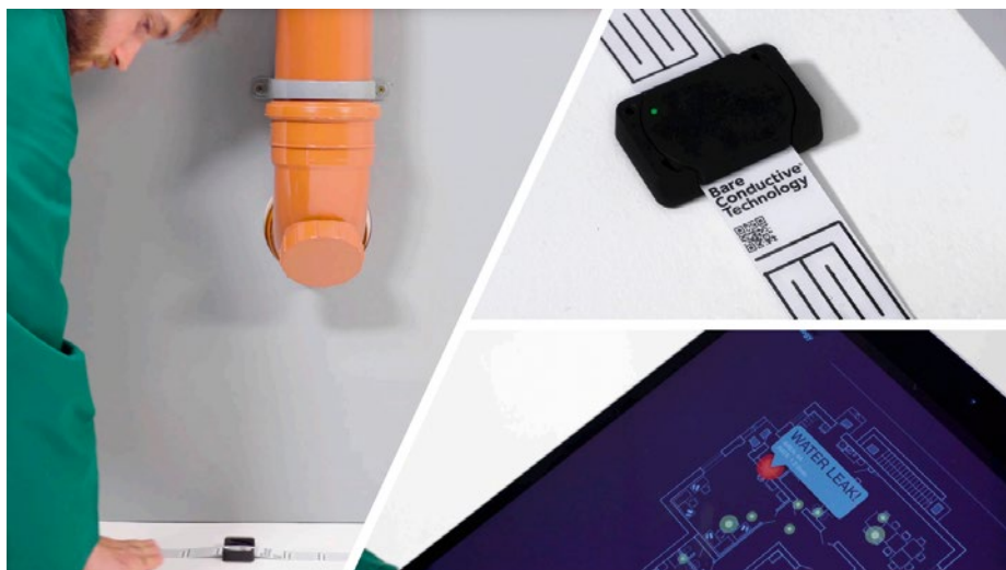
Fig 3: Thin and flexible printed electronics allow for applications in both tight areas as well as non-flat surfaces, such as leaking detection for piping
