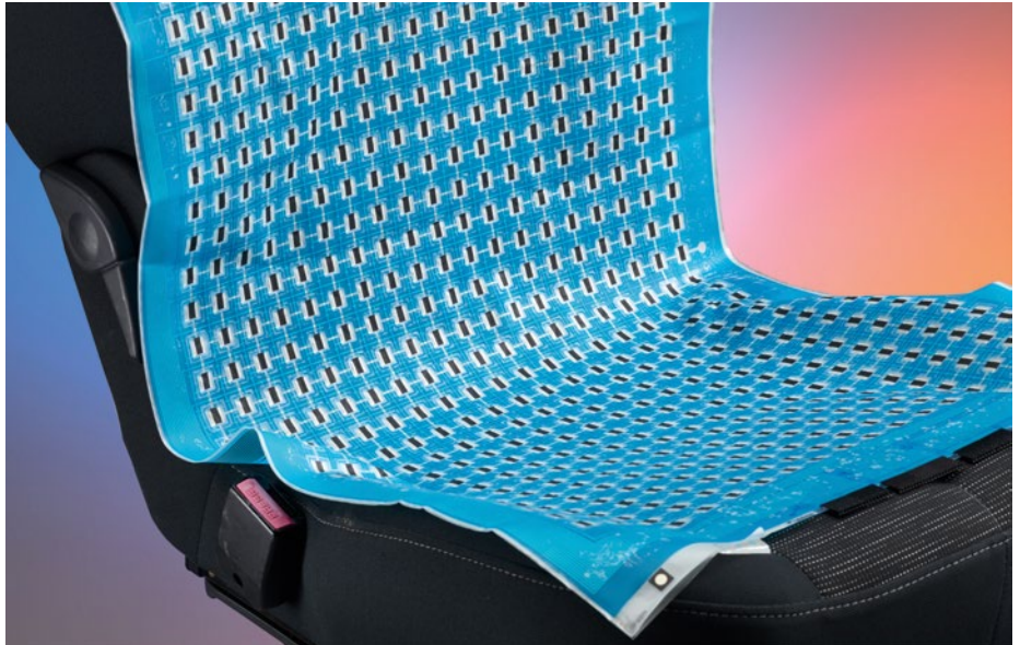
A sensor mat that can be integrated in a car seat
