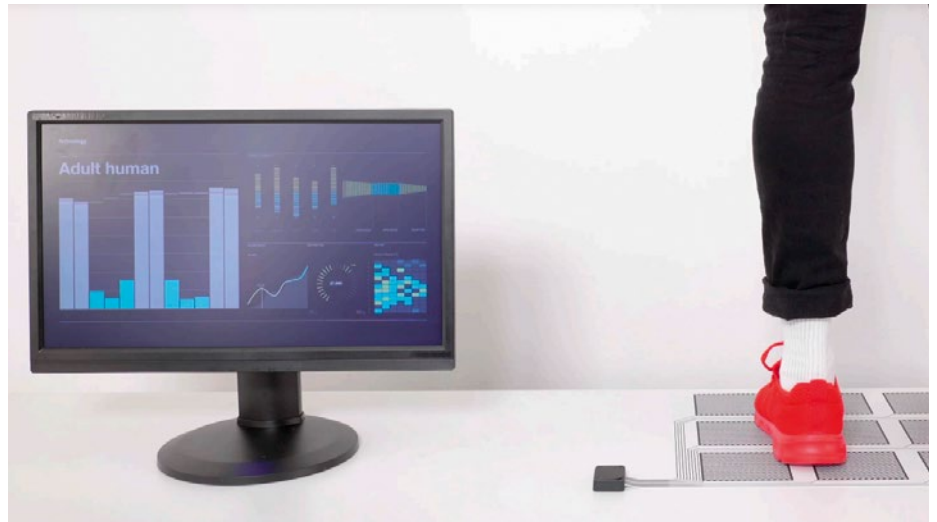
Fig 2: Printed electronics for force sensing flooring surfaces allow for a broad range of new applications – from optimised heating to security functions
