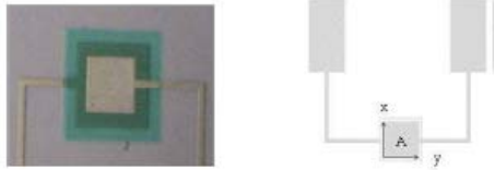
Figure 1. Printed temperature sensor and layout
